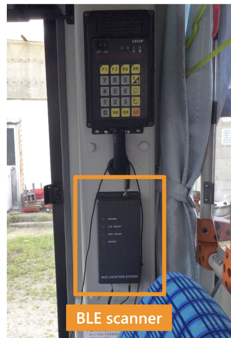
FIGURE 2. BLE scanner for route buses integrated into the bus location system.
