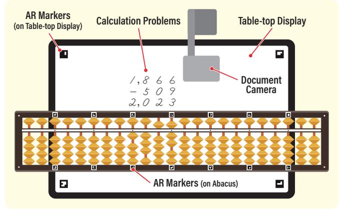
Fig. 2. Design of a table-top interface.
