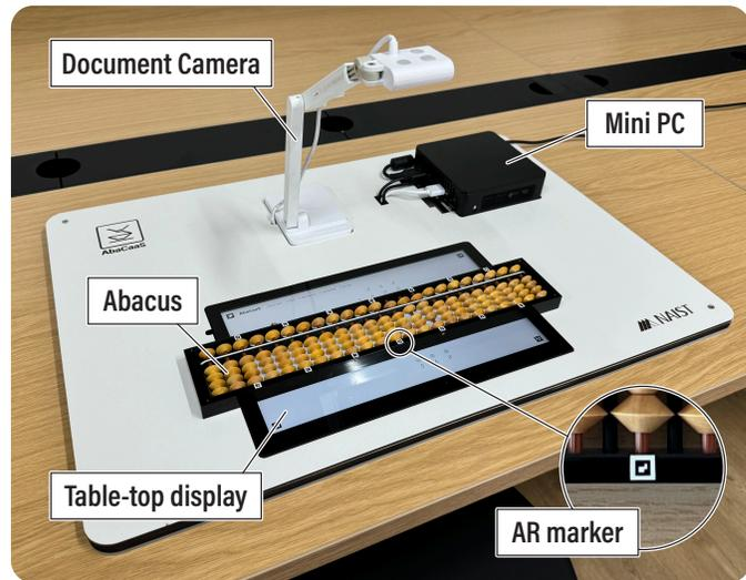
Fig. 1. Abacus learning support system using table-top display and document camera as a sensor (AbaCaaS).
